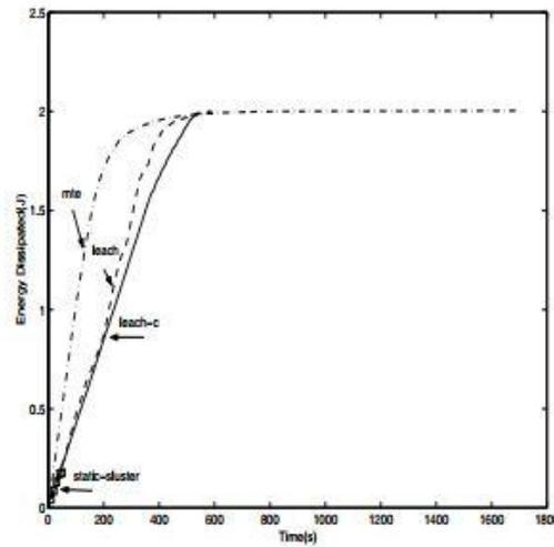
Figure shown above the behaviour of the network in proactive mode. This comparison was originally done in LEACH. It is repeated here taking into account the modified radio energy model. Of the four protocols, mte (minimum transmission energy) lasts for the longest time. However, we observe from Fig that only one or two nodes are really alive. As such, leach and leach-c (a variant of leach) can be considered the most efficient protocols, in terms of both energy
