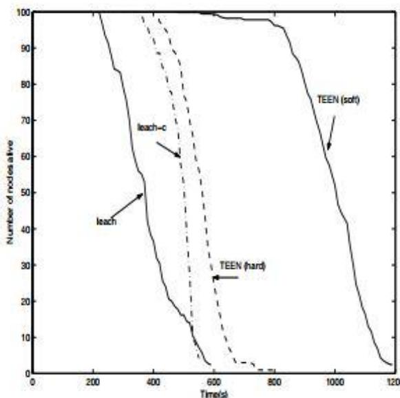
The performance of TEEN is studied in two modes, one with only the hard threshold (hard mode) and the other with both the hard threshold and the soft threshold (soft mode).
